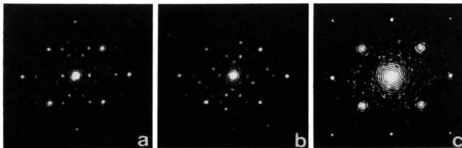
Fig. 7. Selected-area optical diffraction pattern from different areas of the high-resolution image of Fig. 6. (a) Core of the island; a commensurate diffraction pattern is obtained. (b) Boundary region of an island; incommensurate diffraction pattern. (c) The matrix shows the AlTi diffraction pattern only.
